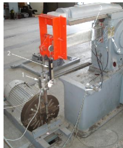
Figure 2 - Main components of fatigue testing system used in experiments
