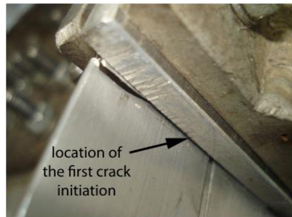
Figure 5 - Location of the first crack initiation
