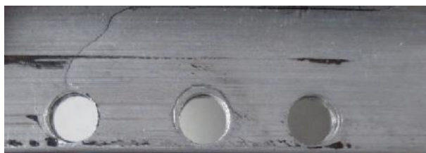
Figure 7 - First crack growth path
