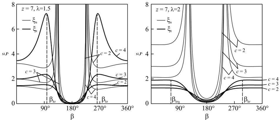
**Fig. 8.** Compared diagrams of the absolute value of the specific sliding of the profile contact point at the trochoidal gear pairs as a function of angle  $\beta$  for the same values of the teeth number by different values of the coefficient  $c$  and for different values of the trochoid coefficient  $\lambda$ : (a)  $z=7, \lambda=1.5$  and (b)  $z=7, \lambda=2$
