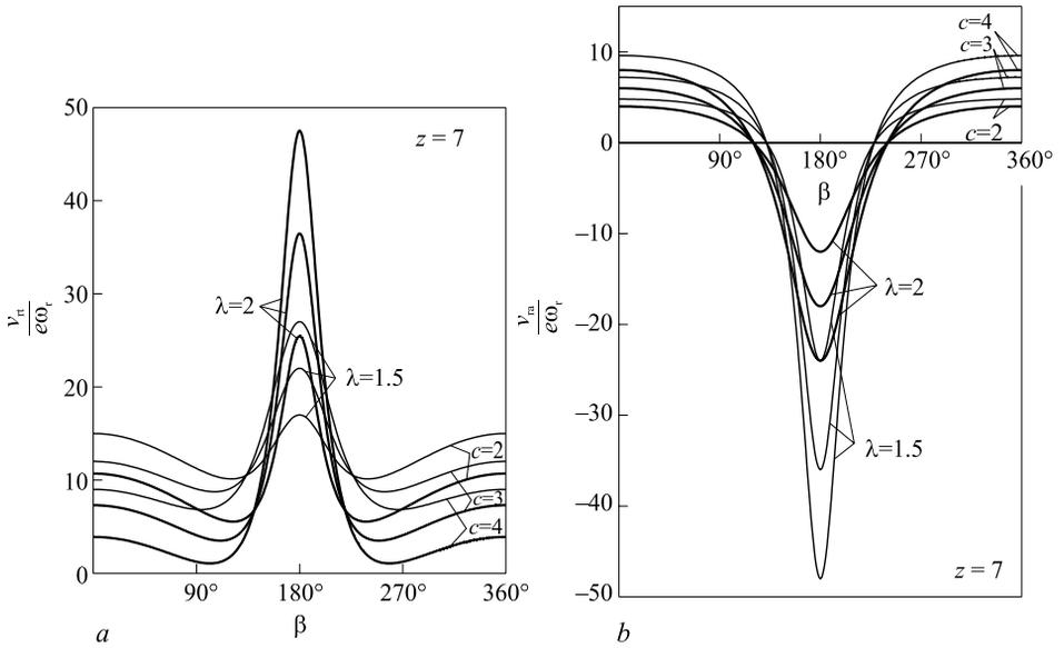
**Fig. 5.** Rolling velocity of the contact point as a function of the angle  $\beta$  for the teeth numbers  $z=7$ , at different values of the coefficient equidistance  $c$  and the trochoid coefficient  $\lambda$ : (a) modified trochoidal profile, and (b) circular profile
