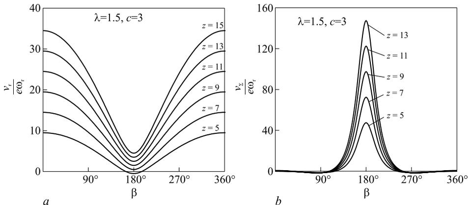
**Fig. 7.** Sliding velocity  $v_t$  of the contact point of the trochoidal profile (a) and summary rolling velocity  $v_\Sigma$  as a function of angle  $\beta$  for the different teeth numbers  $z$  (b), by the trochoid coefficient  $\lambda=1.5$  and coefficient equidistance  $c=3$
