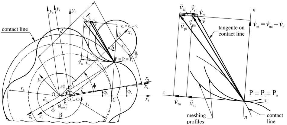
**Fig. 1.** Geometrical and kinematical parameters of the trochoidal gear pair
