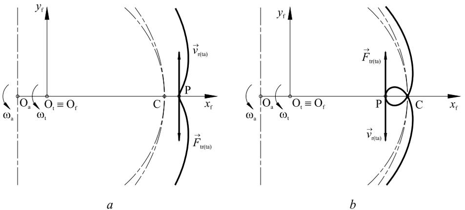
**Fig. 2.** Direction of the sliding velocity and friction force in the contact point P on the referent line at the different form of the contact line of the trochoidal gear pair
