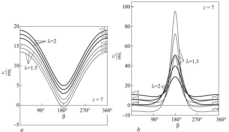
**Fig. 6.** Sliding velocity  $v_r$  of the trochoidal profile (a) and summary rolling velocity  $v_s$  as a function of the angle  $\beta$  for teeth numbers  $z=7$  (b), by different values of the coefficient equidistance  $c$  and trochoid coefficient  $\lambda$ .
