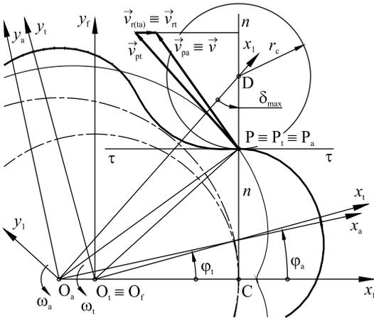
**Fig. 4.** Polygon of velocities in singular contact point
