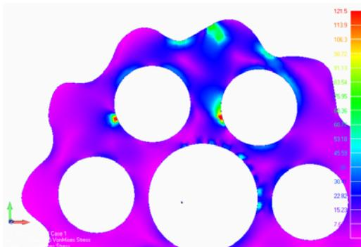
Fig. 7. Von-Mises stress distribution for the case of single meshing when force  $F_{N1}$  is decomposed into three components
