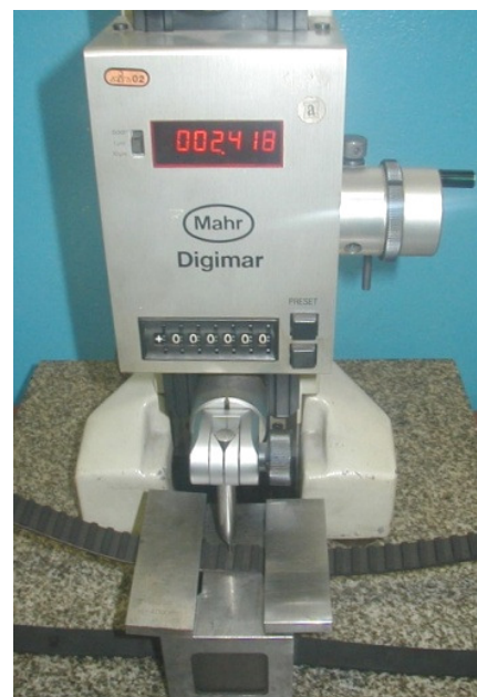
Figure 8. Device for measuring of geometrical dimensions – DIGIMAR
