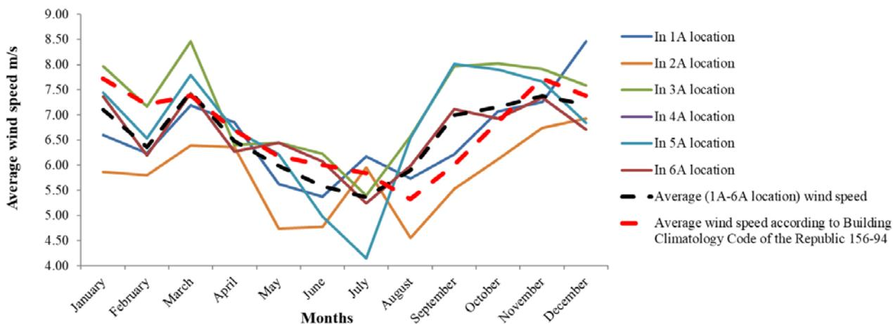
Fig.10. Wind speed in (>1) MW capacity wind turbines/farms
