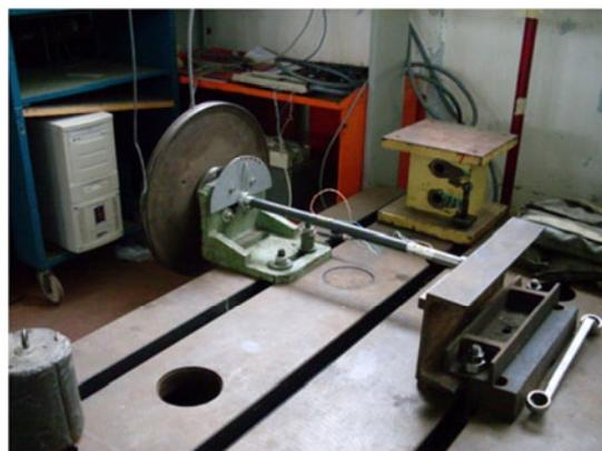
**Fig. 8** The laboratory device for shaft torsion testing
