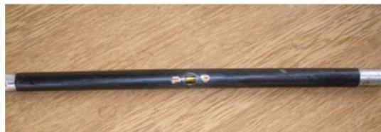
**Fig. 7** The shaft model with glued strain gauges
