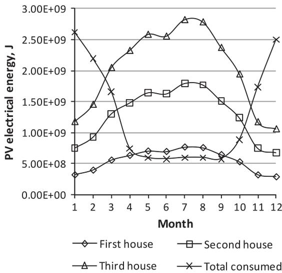
Fig. 8. Monthly values for the generated PV electrical energy by all three houses. The monthly values of the total electrical energy consumed by the houses are given for comparison.
