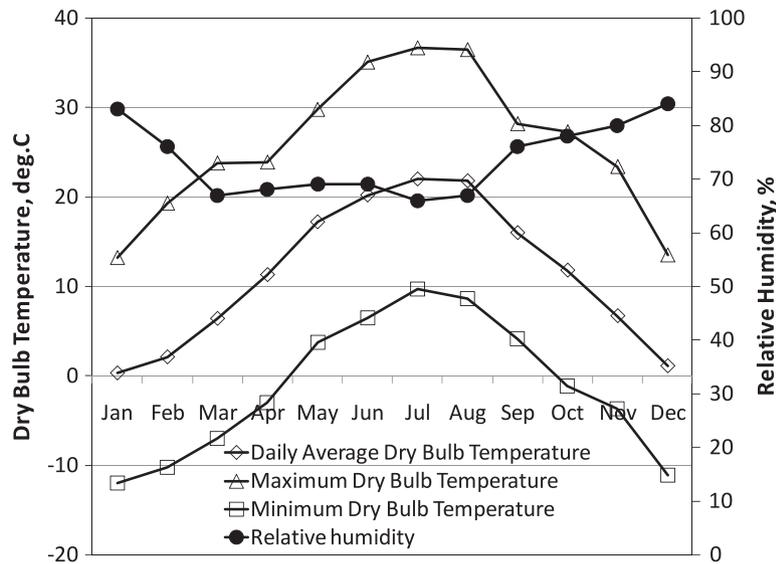
Fig. 2. Relative humidity and dry bulb temperature (minimum, daily average and maximum) from the monthly statistics for Kragujevac, Serbia from Meteororm weather file.
