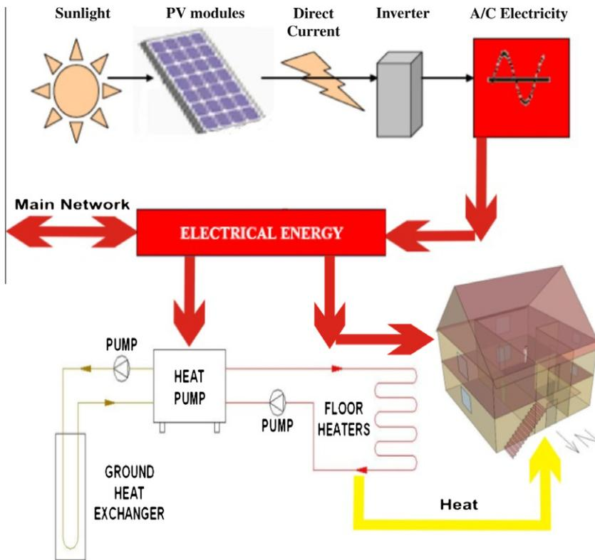
Fig. 1. The house, its heating system, and PV system under investigation (the PV array is located at the house roof facing south).
