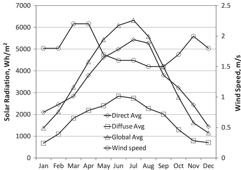
Fig. 3. Direct, diffuse, and global average solar radiation, and daily average wind speed from the monthly statistics for Kragujevac, Serbia from Meteornorm weather file.
