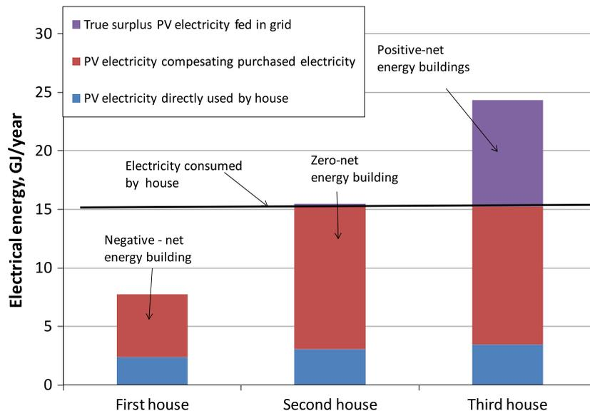
**Fig. 11.** Different types of electrical energy in the houses: the electrical energy consumed by the house, the PV electrical energy directly used in the house, the PV electrical energy compensating purchased electrical energy, and the true surplus PV electrical energy fed in the grid.
