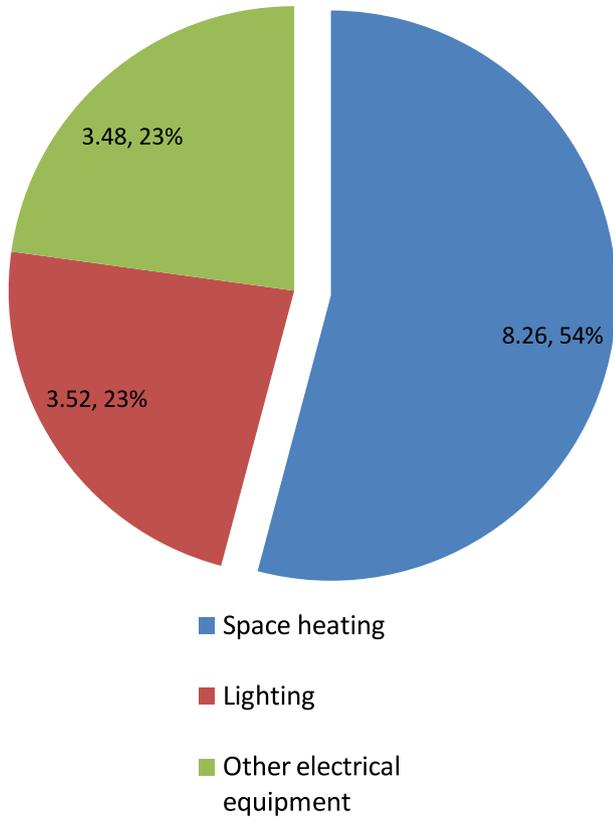
**Fig. 10.** Electrical energy (GJ/year) consumed in the houses: for space heating, for lighting, and by other electrical equipment. The other electrical equipment of this residence is appliances and DHW heating devices.
