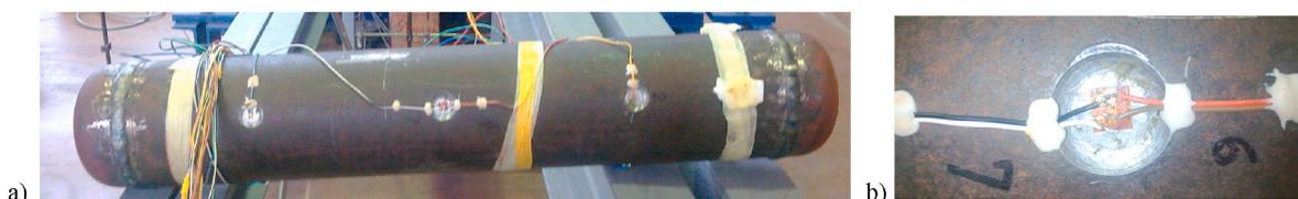
**Fig. 2.** Pipe prepared for the pressure testing, a) overall appearance, b) simulated defects on the pipe, with strain gauges mounted.
