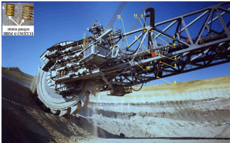
**Fig. 13.** Welded structure of the bucket-wheel boom and spots where strain gauges were located.
