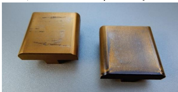
c) contact elements with the TiN coating.
