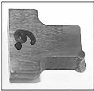
**Fig. 5.** Hard faced shape punch – Sample II (BM-Č4850, FM-Č4850)
