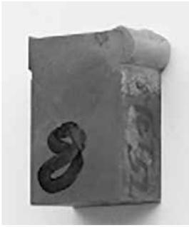
**Fig. 9.** Hard faced shape punch – Sample IV (BM- Č4172, FM- Castolin EUTELLOY 10494)
