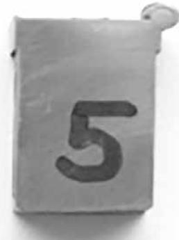
**Fig. 3.** Hard faced shape punch – Sample I (BM-Č4850, FM-Č4172)
