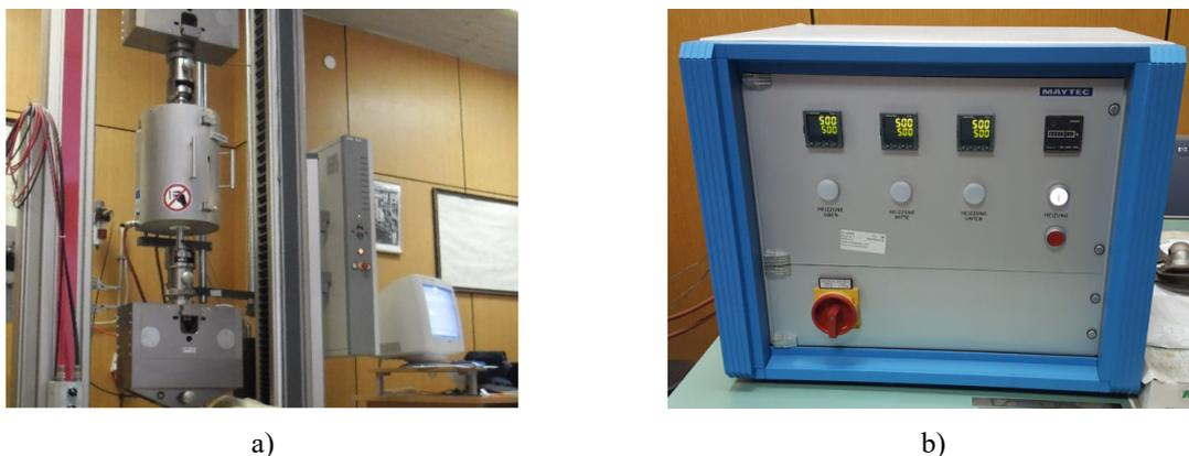
Fig. 3 Testing machine (a) and unit for control of testing temperature (b)
