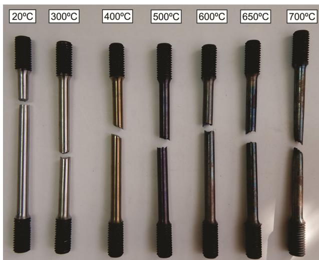
**Fig. 5** Failure modes of H11 steel specimens at elevated temperatures
