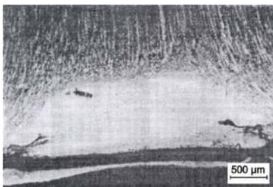
**Figure 6** Micro structure: (a) dynamically recrystallized zone; (b) zone immediately next to the friction plane – forming of the sub-grains within the large austenitic grains (500×)
