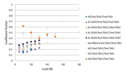
**Fig. 2.** The effect of load on coefficient of friction of the Al/SiC/Gr composites with different weight percentage of SiC particles and fixed 5 wt % Gr [21-24].
