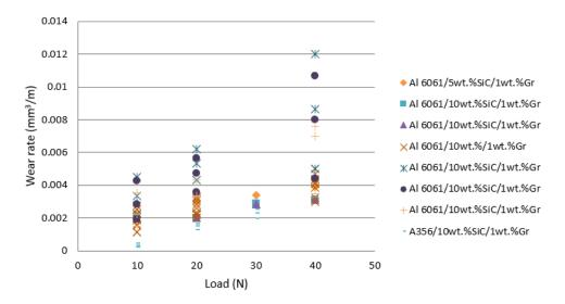
Fig. 1. The effect of load on the wear rate of the Al/SiC/Gr composites with different wt % of the SiC particles and fixed 1 wt % Gr [13, 19-20].
