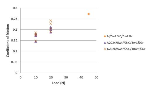
**Fig. 3.** The effect of load on coefficient of friction of the Al/SiC/Gr composites with different wt % of the Gr particles and fixed 5 wt % SiC [15, 25].
