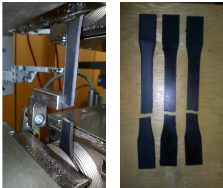
Fig. 2. Broken specimen in the machine grips (left) and three specimens after tensile test (right).
