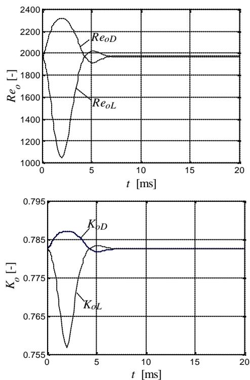
**Figure 6** Time dependences of Reynolds number and flow coefficient of left and right constant orifice
