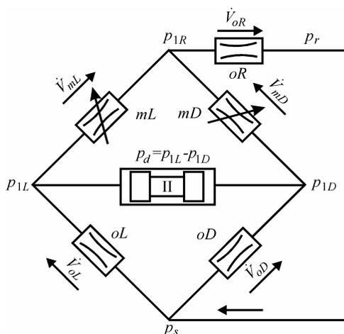
**Figure 1** Scheme of the first stage of hydraulic amplification
