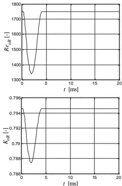
**Figure 7** Time dependences of Reynolds number and flow coefficient of drain orifice
