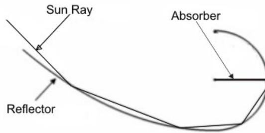
Figure 5 Solar ray path toward the concentrator with 4 reflections (the cross cut of parabolic-cylindric concentrator).
