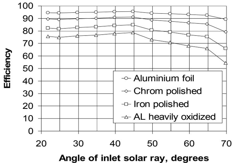
Fig. 7 Efficiency of use of solar rays at reflector
