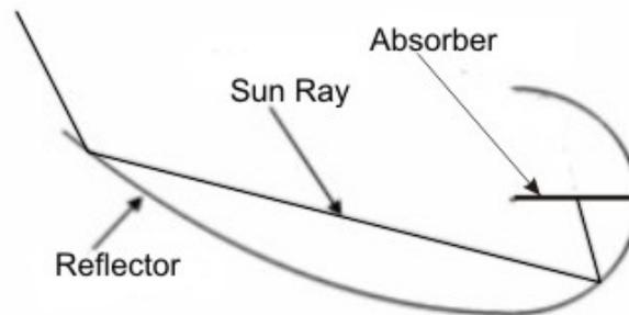
Figure 4 Solar ray path toward the concentrator with two reflections from reflector (the cross cut of parabolic-cylindric concentrator).
