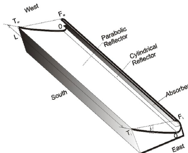
Figure 1 Position of the concentrator of CP-90A type.
