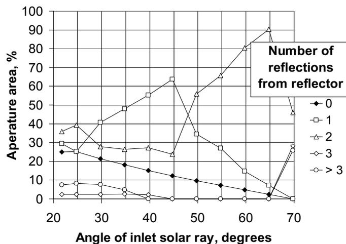
Figure 6 Aperture area as a function of inlet angle of solar ray
