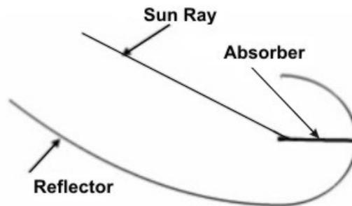
Figure 3 Solarray path toward the concentrator that hits the absorber directly (the cross cut of parabolic-cylindric concentrator).
