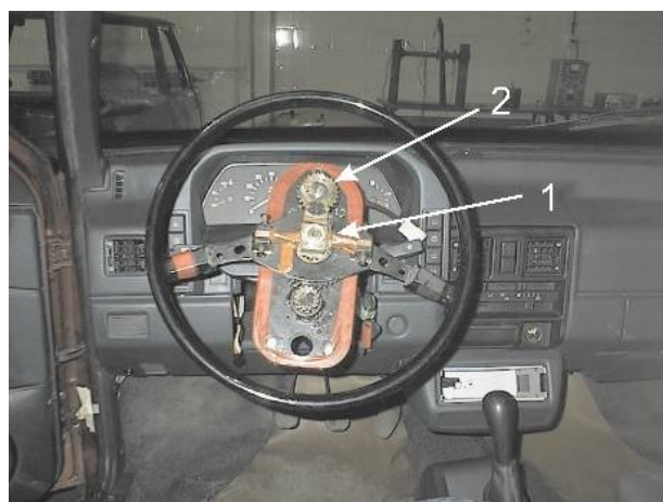
Figure 2. Dynamometric steering wheel for measurement of the steering wheel torque and the steering wheel angle [31].
