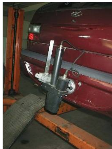
Figure 5. Correlation-optical sensor for measurement of vehicle longitudinal speed.
