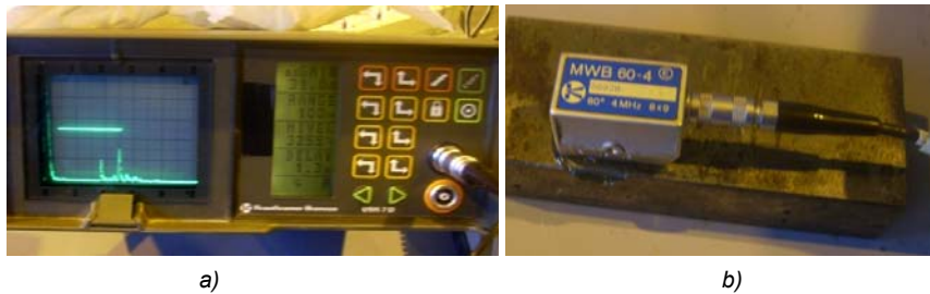
Fig. 9. Ultrasonic testing: a) Ultrasonic testing device; b) Testing probe
