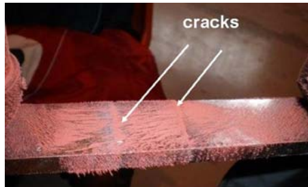
Fig. 6 Magnetic particle nondestructive testing method
