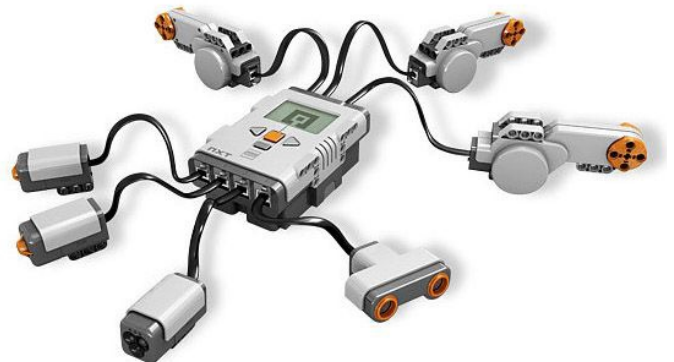
Fig. 1. LEGO Mindstorms NXT 8540: programmable unit, three DC motors with integrated encoders, two touch sensors, color/light sensor, and ultrasonic distance sensor.
