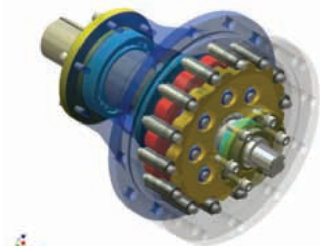
Figure 1. Model of a single-stage cycloid drive
