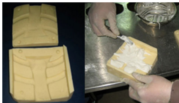
Fig. 14 Upper and lower plates of the casting mold ( left ) and filling the mold cavity with prosthetic material ( right )
