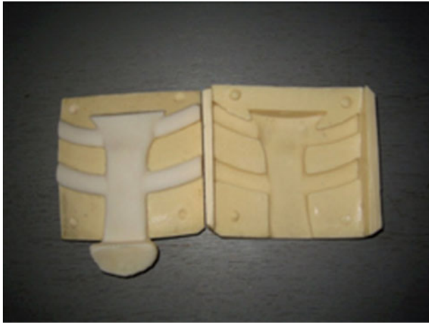
Fig. 15 Implant in the lower casting mold plate before removing and post processing
