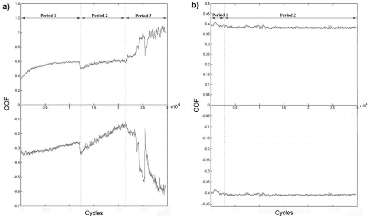
**Figure 4.** Averaging of the envelope signal of COF curve: a)  $v=4$  mm/s;  $F_N=100$  mN; b)  $v=12$  mm/s;  $F_N=1000$  mN
