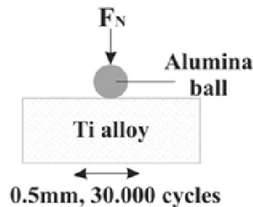
**Figure 1.** The scheme of the contact pair geometry
