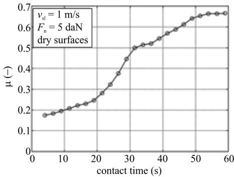
**Fig. 14.** Friction coefficient as a function of time
