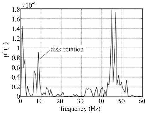
**Fig. 7.** Power spectrum of the friction coefficient after the contact duration time of 54 min and 40 s
