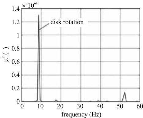
**Fig. 5.** Power spectrum of the friction coefficient after the contact duration time of 20 min
