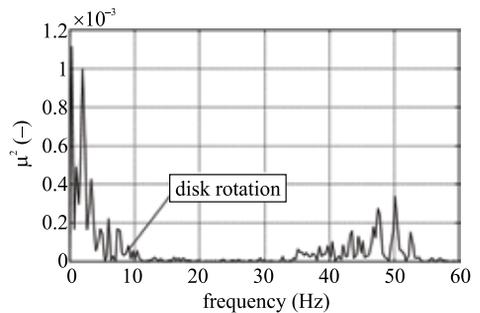
**Fig. 17.** Power spectrum of the friction coefficient in the period 45–48 s
