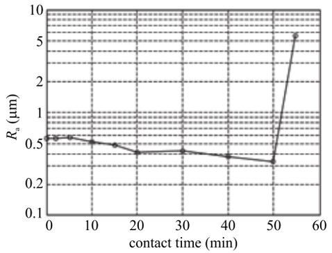
**Fig. 8.** Variation of the disc average roughness with contact duration time
