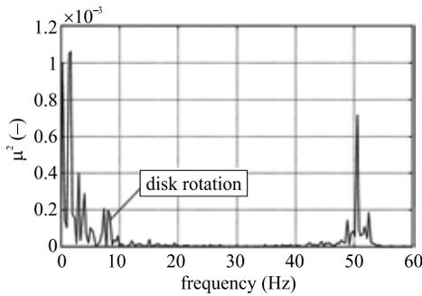
**Fig. 16.** Power spectrum of the friction coefficient in the period 21–24 s
