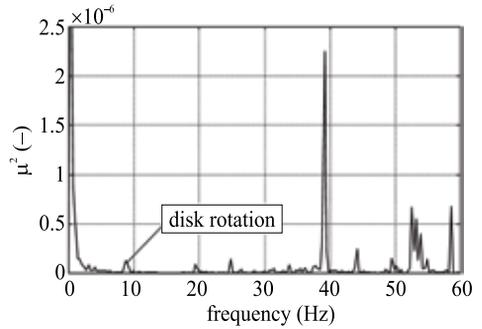
**Fig. 15.** Power spectrum of the friction coefficient in the period 2–5 s
