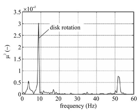
**Fig. 6.** Power spectrum of the friction coefficient after the contact duration time of 54 min and 20 s
