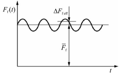
Fig. 1. Idealised form of the friction force
