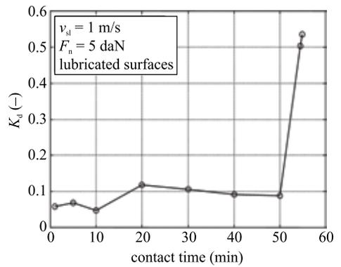
**Fig. 4.** KDB as a function of contact duration time
