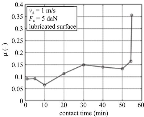
**Fig. 3.** Friction coefficient as a function of contact duration time
