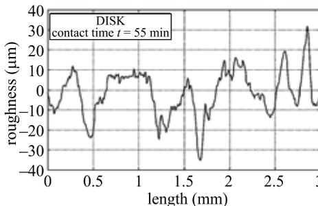
**Fig. 13.** Surface topography ( $t = 55$  min)
