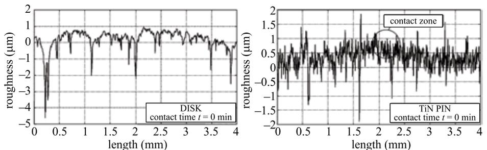
**Fig. 9.** Surface topography ( $t = 0$  min)
