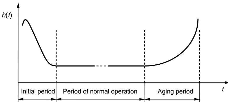
**Figure 1.** The intensity of failure of mechanical systems' elements as a function of operating time
