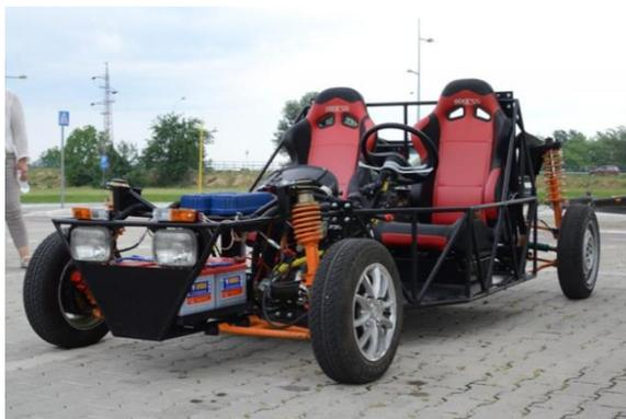
**Figure 1.** Hermes, hybrid-electrical vehicle [1]
