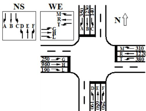
**Figure 2.** Test intersection with phase plan and traffic demands
