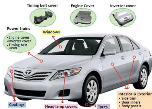
**Figure 2.** Illustration of the usage of polymer nanocomposites parts [6]
