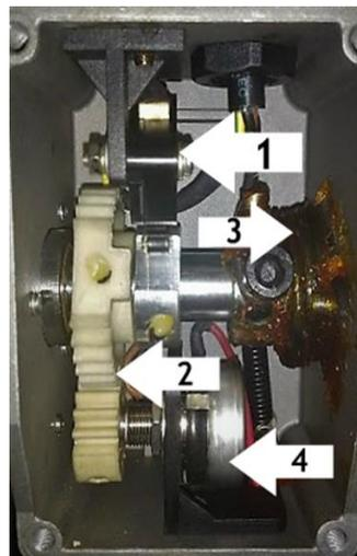
**Figure 3.** Main parts of acceleration pedal's mechanism
