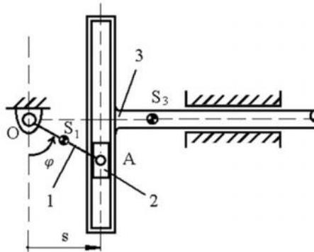
**Figure 7.** Working principle of a Scotch yoke mechanism [6]
