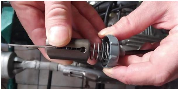
**Figure 5.** Complete appearance of the needle throttle valve
