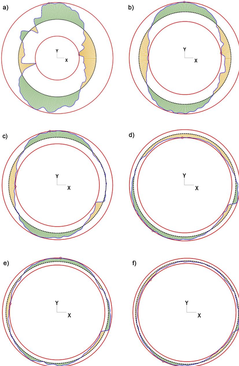
**Fig. 10.** Plots of the roundness deviations, (a) opening 1, (b) opening 2, (c) opening 3, (d) opening 4, (e) opening 5, (f) opening 6. (For interpretation of the references to colour in this figure caption, the reader is referred to the web version of this article.)
