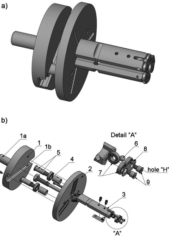
**Fig. 8.** Ball burnishing tool, (a) CAD model, and (b) exploded view.
