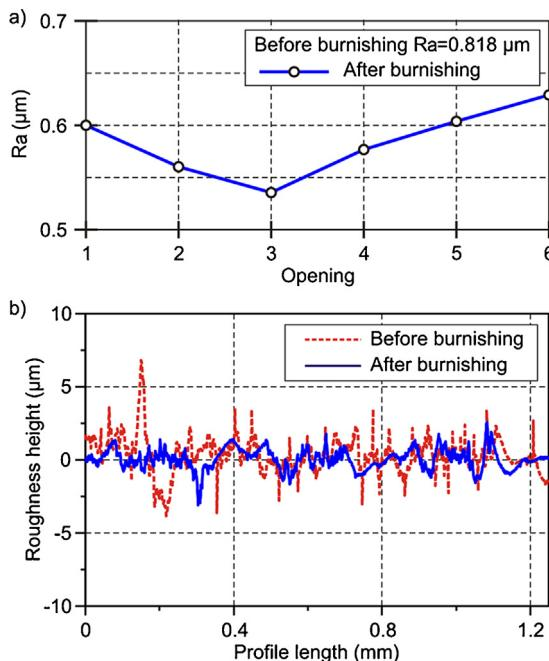
**Fig. 11.** Roughness, (a) diagram of the  $R_a$  variation for openings 1–6 and (b) the overlapped surface roughness profile before burnishing and roughness profile of opening 3 after ball burnishing.
