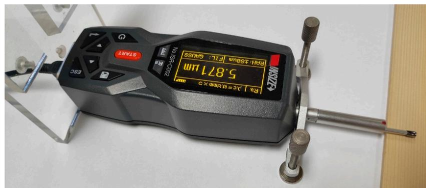
**Figure 6.** Surface roughness measurement.
