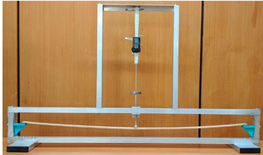
**Figure 5.** Elastic modulus measurement.
